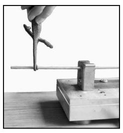
FIG. 1. Picture illustrating the set-up used to measure tail-gripping performance for *Bradypodion pumilum*. The chameleon is allowed to wrap its tail around the dowel mounted onto the force plate and is then pulled dorsally.
